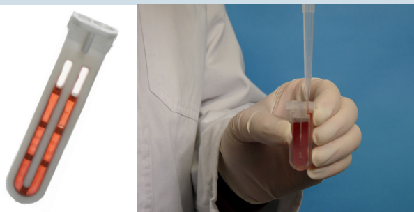
Both, MD100/300 (left) and MD 1000 dialyzer devices are easy to load using a standard micropipette.
